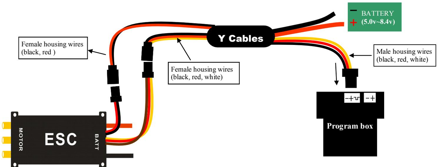
**NOTE:** When connect 300A ESC to Program box, please DO NOT connect ESC to motor and main
